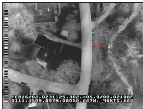
Figure 72: Aerial thermography showing sewage leak
