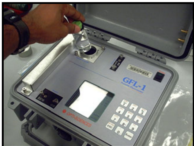
Figure F3.5: Placing Sample into Sample Chamber
